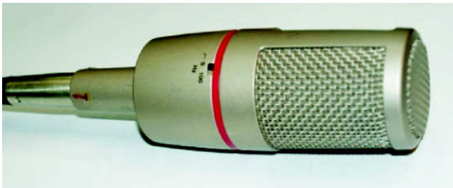
Figure 13.2: A condenser microphone. (Source: Jnan Taranga, KKHSOU, Guwahati)
