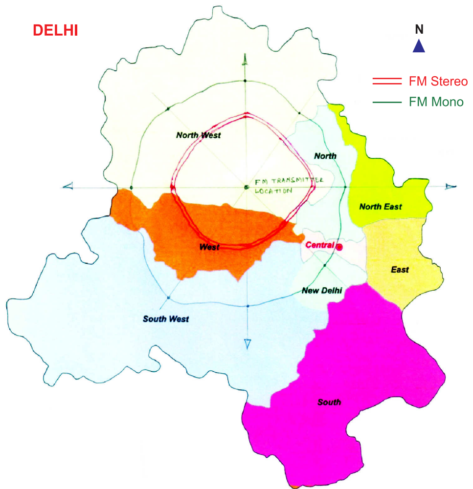
Figure 26.8: Actual coverage map of a 300 w FM transmitter
