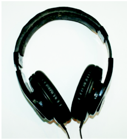
Figure 13.11: A pair of over-the-ear headphones. Note the cups that cover the entire ear. (Source: Jnan Taranga, KKHSOU, Guwahati)
