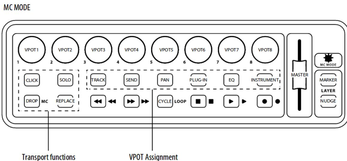
Fig. 62.10 - X-Touch Mini MC mode layout
