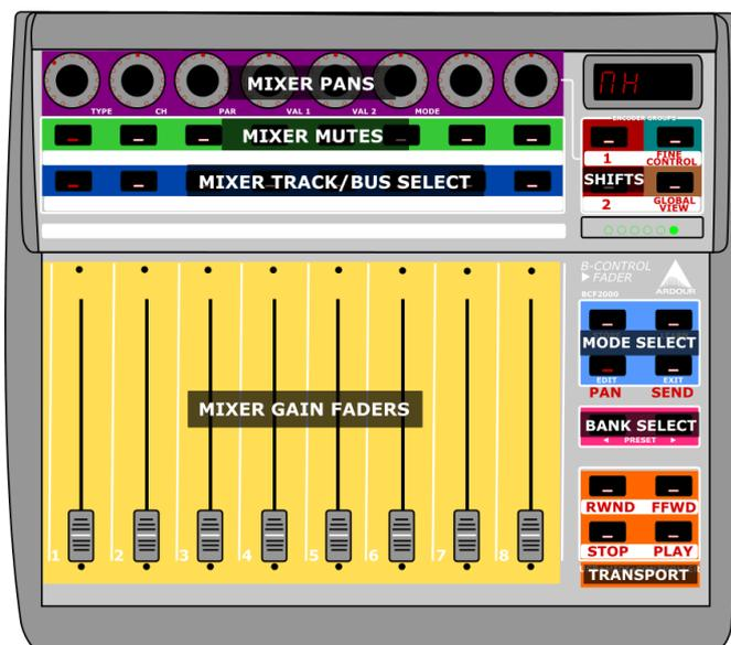
Fig. 62.5 - Diagrammatic Image of the BCF2000 Control Modes (click for a full-size view)
