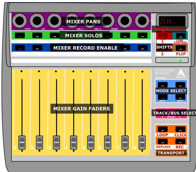
Fig. 62.7 - Diagrammatic Image of the Mixer Mode while holding down Shift 1
