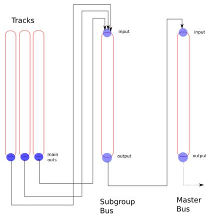
Fig. 54.5 - Sub group signal routing
