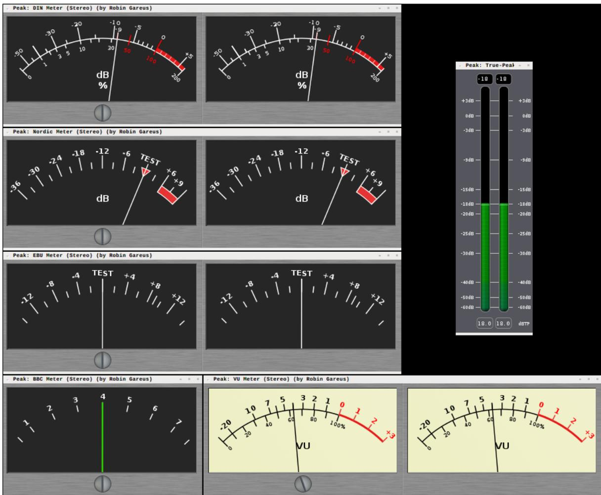
Fig. 54.3 - Needle-style meters as external LV2 plugins
