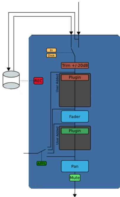
Fig. 54.7 - Typical signal routing in a channel strip.
