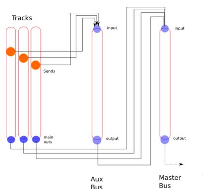
Fig. 54.4 - Aux signal routing
