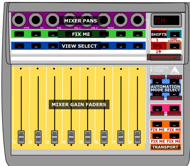
Fig. 62.8 - Diagrammatic Image of the Mixer Mode while holding down Shift 2
