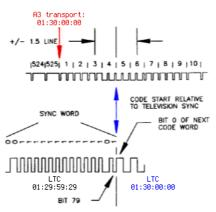
Fig. 7.3 - LTC frame alignment for the 525/60 TV standard
