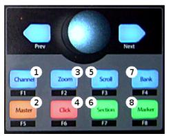
Fig. 65.3 - FaderPort8 Navigation Buttons
