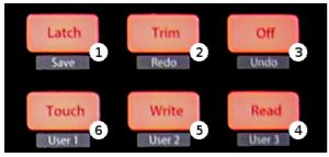
Fig. 65.8 - FaderPort8 Automation Buttons
