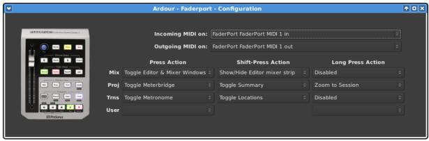
Fig. 64.1 - The Faderport configuration dialog
