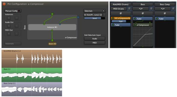
Fig. 54.10 - A sidechain compression: Pin configuration, mixer view and editor view.
