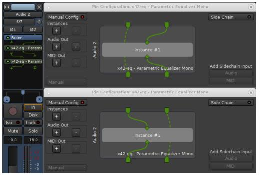
Fig. 54.9 - An example of using two mono plugins on a stereo track.
