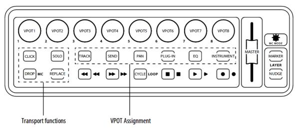
Fig. 62.10 - X-Touch Mini MC mode layout
