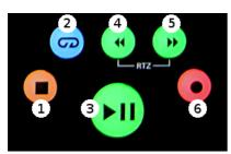
Fig. 65.2 - FaderPort8 Transport Buttons
