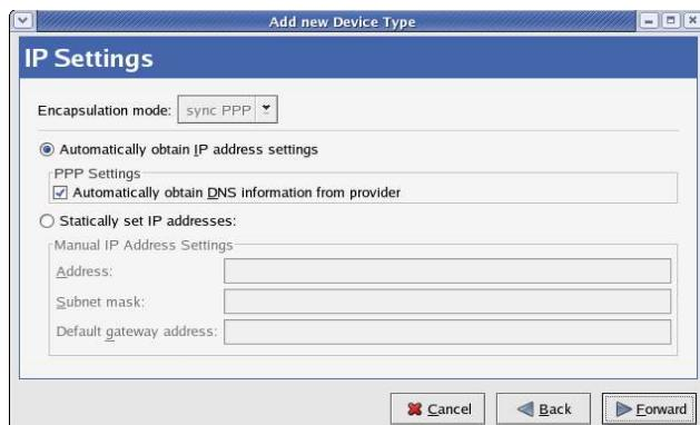
**Fig. Filling in the IP Settings**
